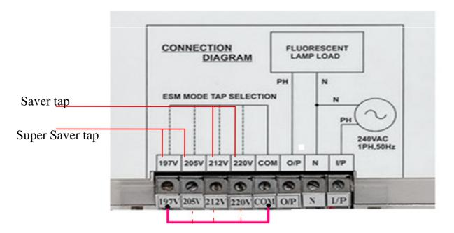
**Step 2:** Keep the AOB switch to overall bypass position. Switch the MCB to ON position. Turn on mains supply and check that all lamps load are in on condition.
